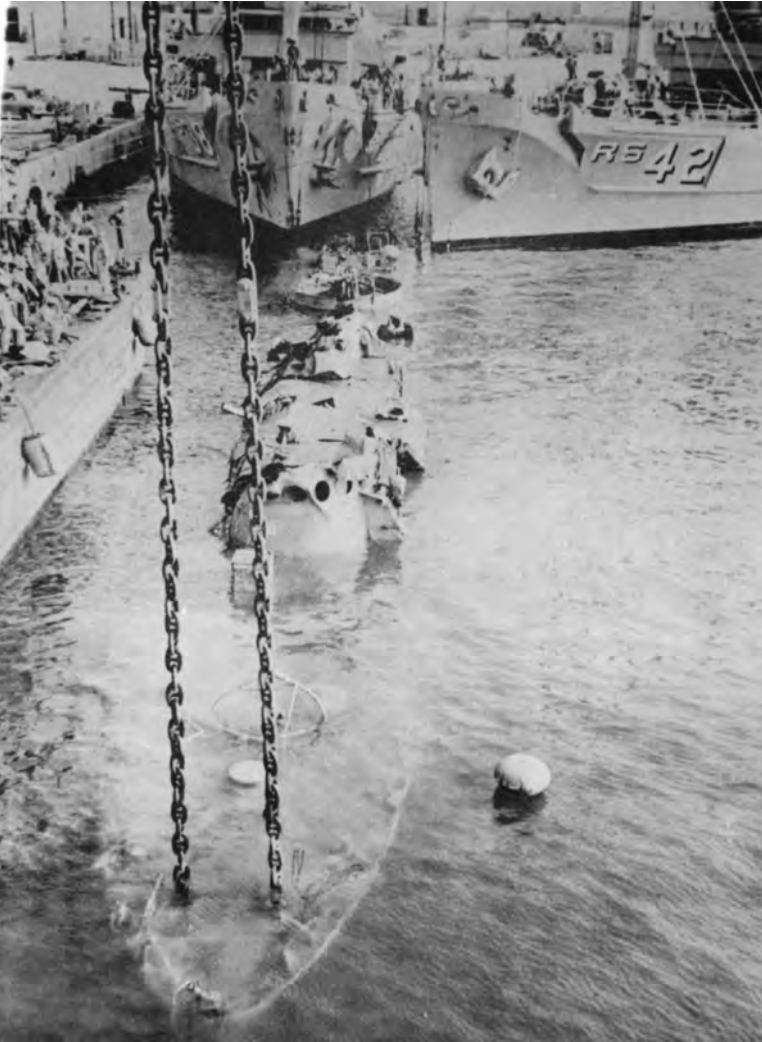
The main deck of patrol craft Han Ra San (PC 705) is about to break the surface, lifted by Bolster , Reclaimer , and the crane YD-120.
