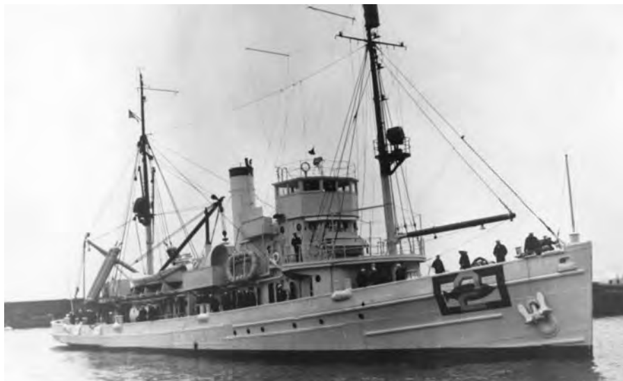
Falcon (ARS 2) was one of six Bird-class minesweepers designated as submarine rescue ships.
