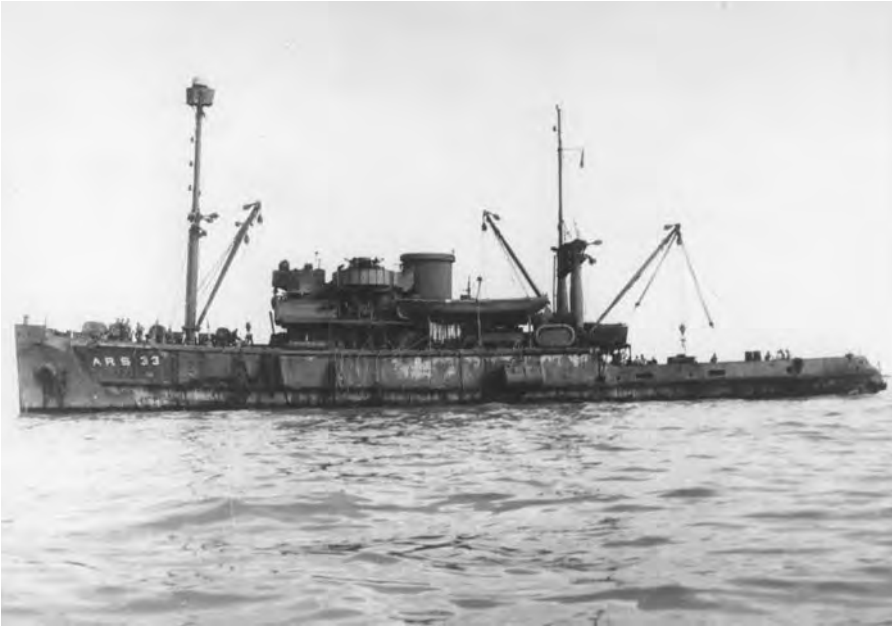
Signs of the sea show plainly on Clamp (ARS 33), the first steel-hulled salvage ship commissioned in the U.S. Navy. The twin kingpost aft is characteristic of ships that were originally BARS.
