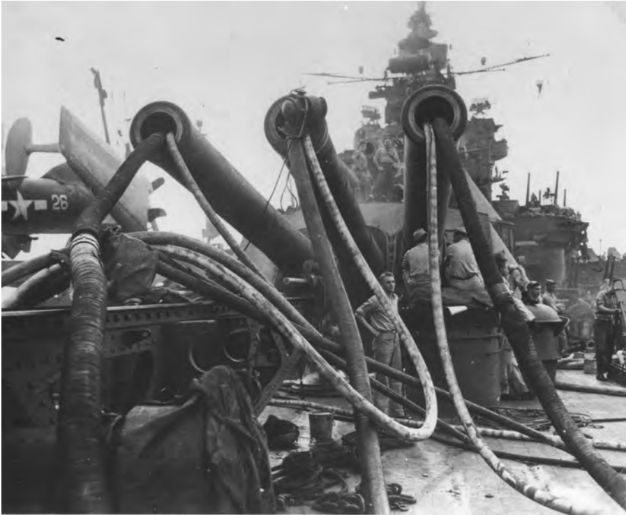
When Pennsylvania was torpedoed at Okinawa, hoses for pumps were run through her 14-inch guns to reach the magazines. The battleship is not shooting hoses. Photo courtesy Captain James W. Greely.
