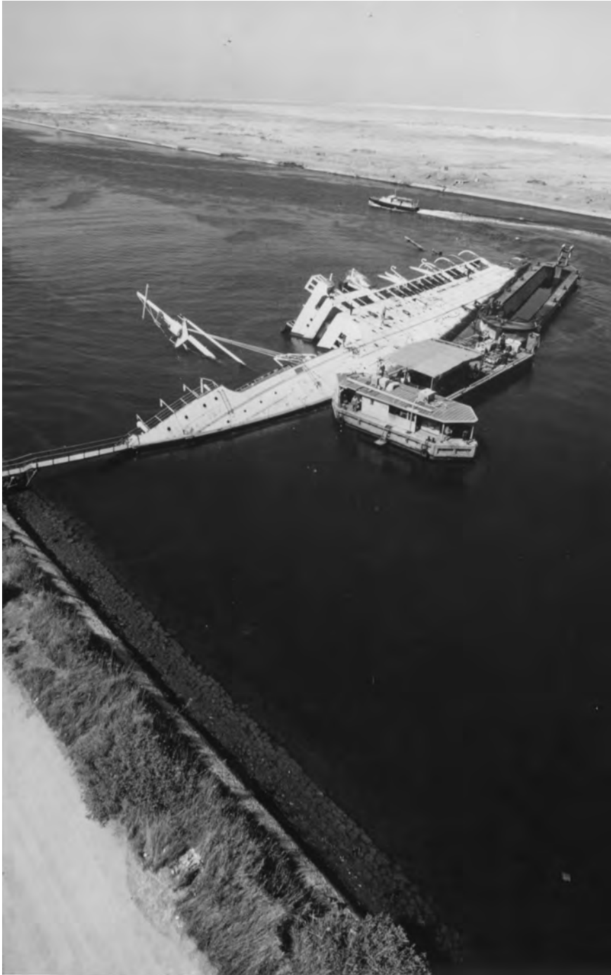
The wreck of the passenger ship Mecca lies athwart the Suez Canal. Mecca was the largest and one of the most formidable obstacles to the 1974 clearance of the canal.
