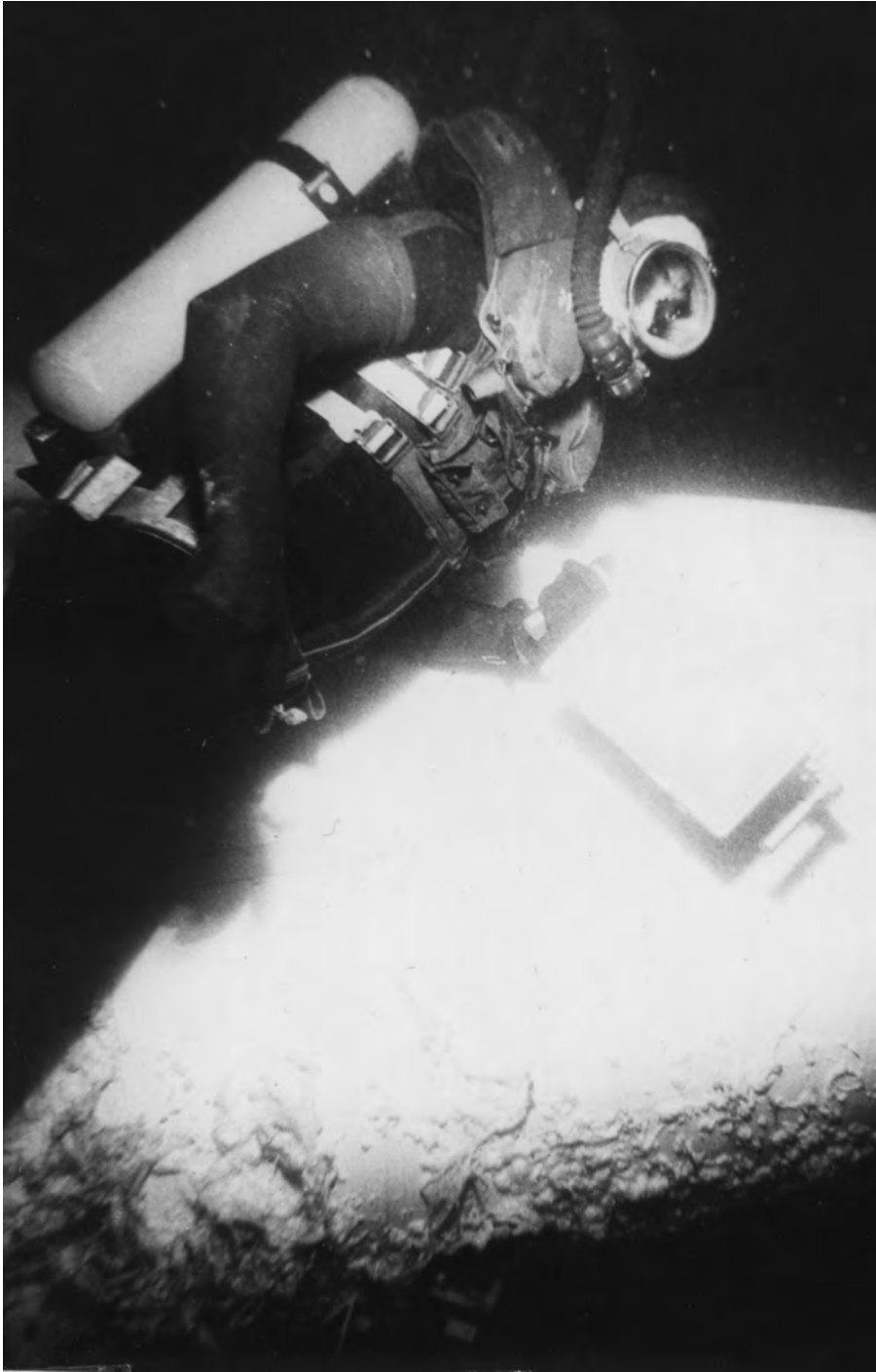
Petty Officer P.A. Wells applies salvage foam to a sunken aircraft during SeaLab II.
