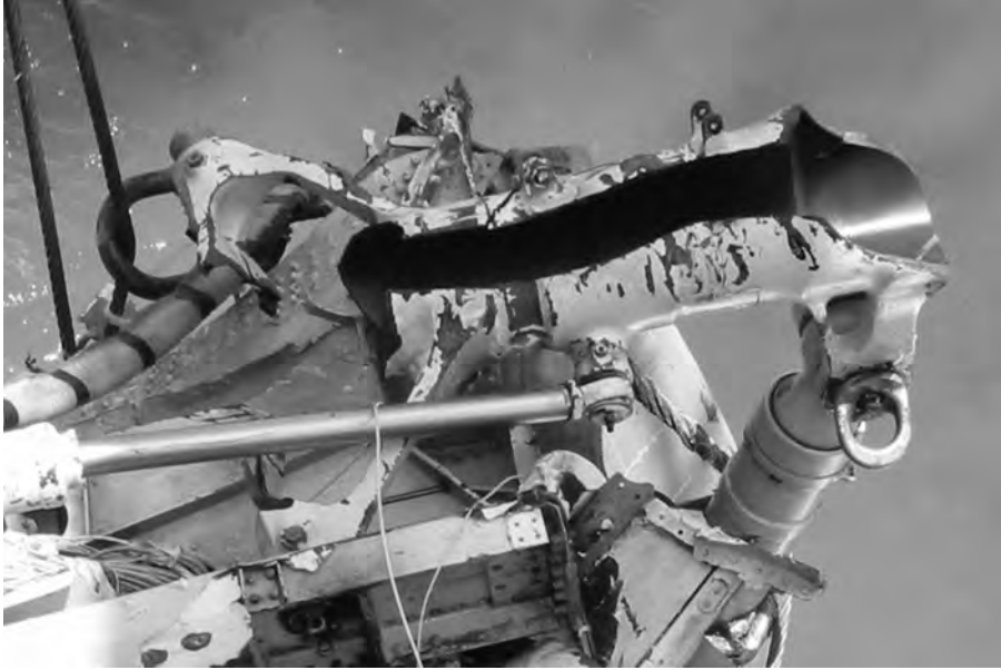
Recovered F-14 nose landing gear cylinder.
