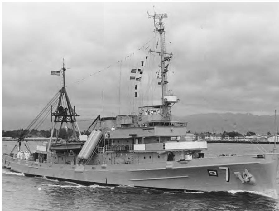
The Chanticleer class were the first purpose-built submarine rescue ships. Chanticleer (ASR 7) appears here as she looked in the early 1960s.
