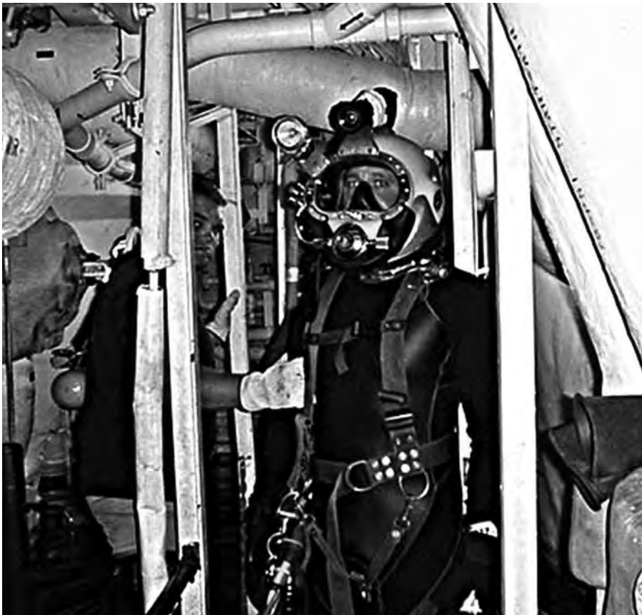
A Navy diver is about to enter Cole's lower-level, flooded engine room through the upper-level gas turbine inlet trunk.
