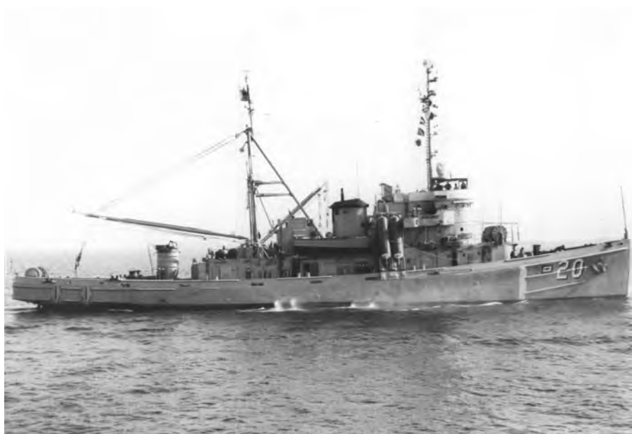
Skylark (ASR 20) was one of three fleet tugs converted to submarine rescue ships. These ships were somewhat smaller and less capable than the Chanticleers .
