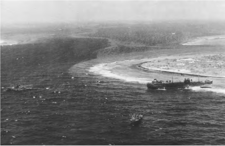
Reclaimer and Beaufort pull on Anangel Liberty, grounded hard on French Frigate Shoal.
