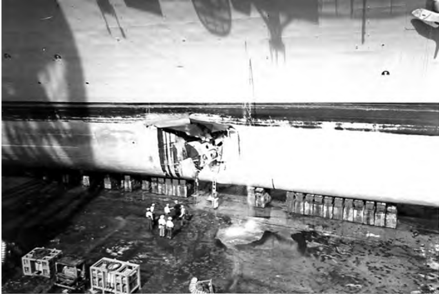
Mine damage on Tripoli's starboard side.
