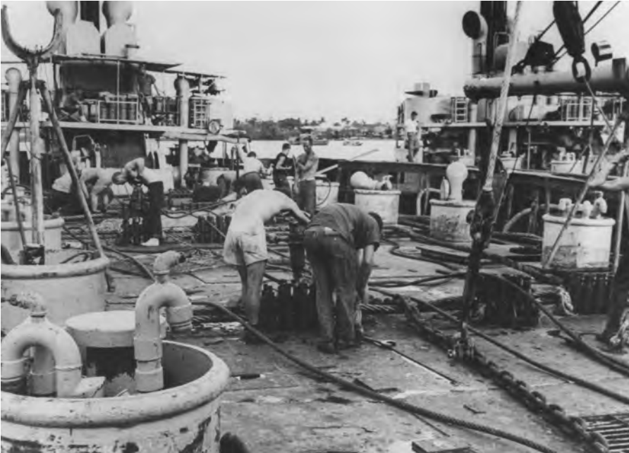
Salvors work “head down, backside up” on deck of their British lift craft during the Paul Bert salvage. The heavy pieces on deck are Bullivant clamps used to clamp the lift wires together. Unlaid manila line in the clamps absorb grease squeezed from the wire and prevent slippage. The clamps are tightened by large pneumatic wrenches called “windy spanners.” Photo courtesy Commander Billie L. Delanoy.
