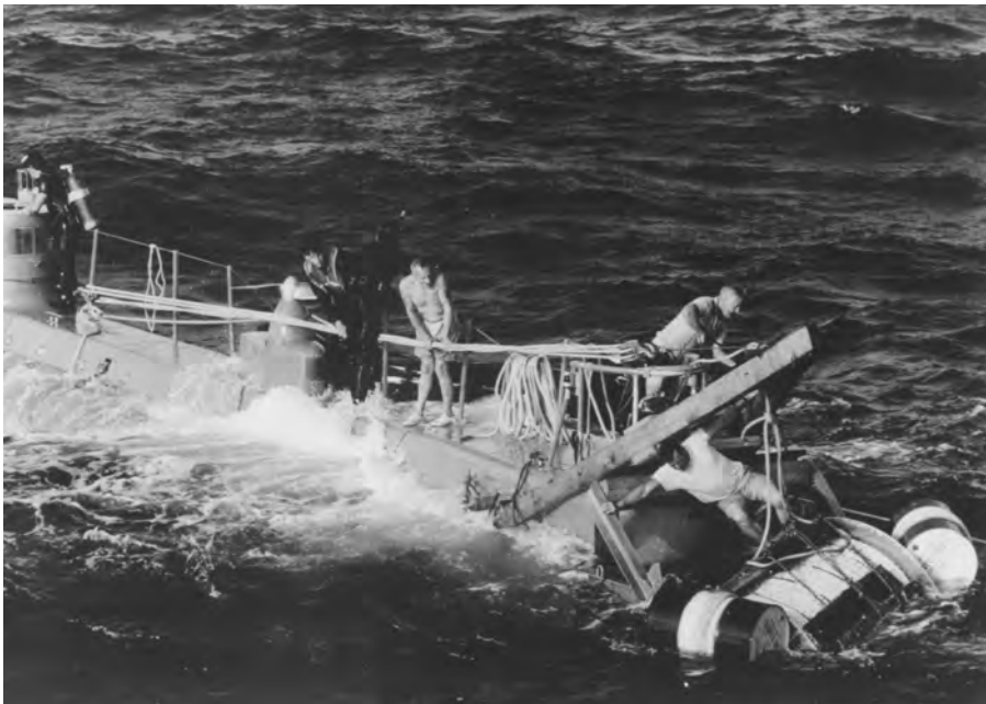
Aluminaut crew and support people work to rig the line reel on the submersible's bow early in the operation that recovered Alvin .
