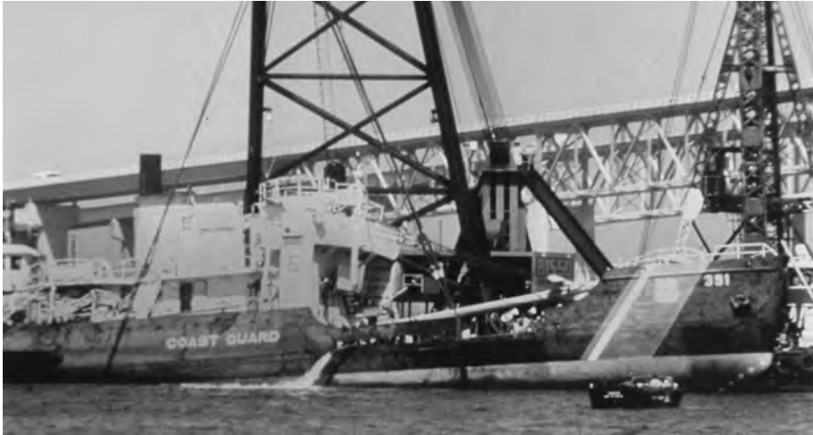
The 650-ton shear leg crane Cappy Bisso lifts the buoy tender Blackthorn from the waters of Tampa Bay, Florida.
